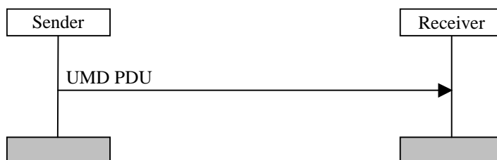
Figure 11.2: Unacknowledged mode data transfer procedure
