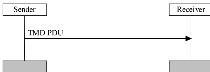
Figure 11.1: Transparent mode data transfer procedure
