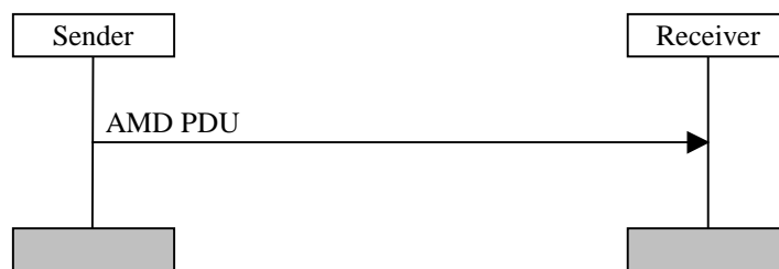
Figure 11.3: Acknowledged mode data transfer procedure
