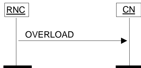
Figure 4: Overload at the UTRAN. Successful operation.
