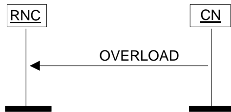
Figure 3: Overload at the CN. Successful operation.
