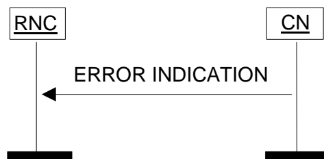
Figure 7: Error Indication procedure, CN originated. Successful operation.
