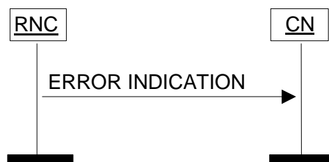
Figure 8: Error Indication procedure, RNC originated. Successful operation.
