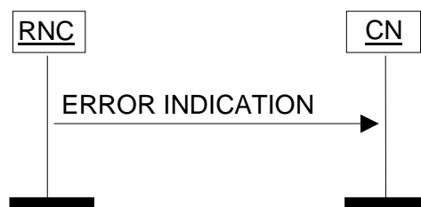
Figure 8: Error Indication procedure, RNC originated. Successful operation.
