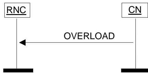
Figure 3: Overload at the CN. Successful operation.
