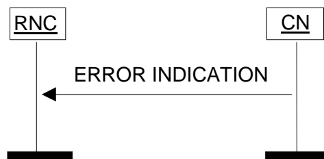
Figure 7: Error Indication procedure, CN originated. Successful operation.
