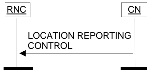
Figure 1: Location Reporting Control procedure. Successful operation.
