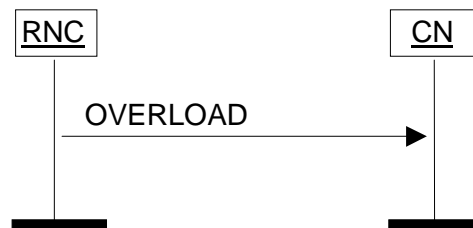
Figure 4: Overload at the UTRAN. Successful operation.
