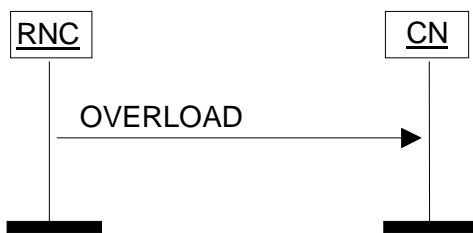
Figure 28: Overload at the UTRAN. Successful operation.
