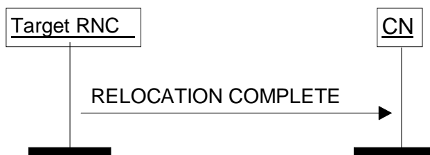
Figure 10: Relocation Complete procedure. Successful operation.
