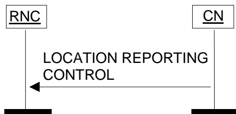
Figure 21: Location Reporting Control procedure. Successful operation.
