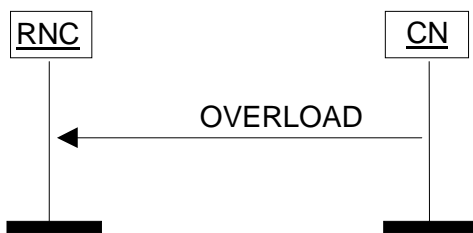
Figure 27: Overload at the CN. Successful operation.
