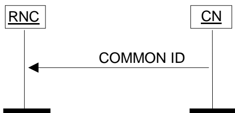
Figure 17: Common ID procedure. Successful operation.
