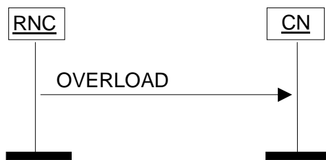
Figure 28: Overload at the UTRAN. Successful operation.
