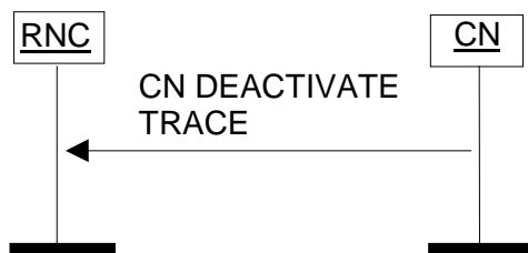
Figure 33: CN Deactivate Trace procedure. Successful operation.
