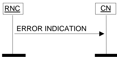
Figure 32: Error Indication procedure, RNC originated. Successful operation.
