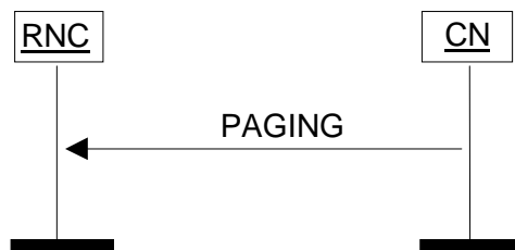
Figure 16: Paging procedure. Successful operation.
