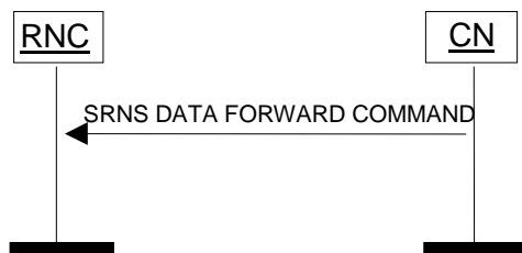
Figure 13: SRNS Data Forwarding Initiation procedure. Successful operation.
