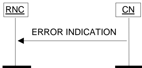
Figure 31: Error Indication procedure, CN originated. Successful operation.
