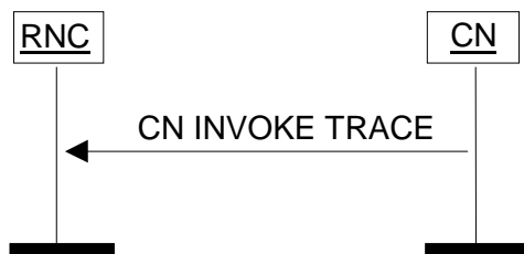
Figure 18: CN Invoke Trace procedure. Successful operation.
