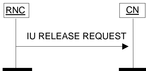
Figure 3: Iu Release Request procedure. Successful operation.
