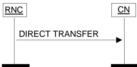
Figure 26: Direct Transfer, RNC originated. Successful operation.
