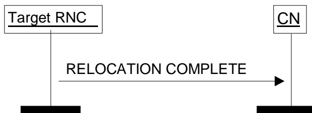
Figure 10: Relocation Complete procedure. Successful operation.
