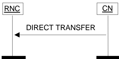
Figure 25: Direct Transfer, CN originated. Successful operation.
