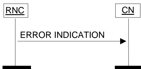
Figure 32: Error Indication procedure, RNC originated. Successful operation.
