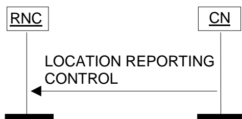
Figure 21: Location Reporting Control procedure. Successful operation.
