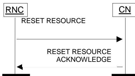
Figure 34: RNC initiated Reset Resource procedure. Successful operation.
