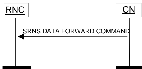
Figure 13: SRNS Data Forwarding Initiation procedure. Successful operation.
