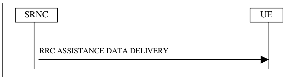
Figure 6.2: OTDOA or GPS Assistance Data Delivery Flow
