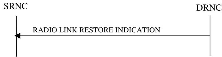
Figure 15: RL Restoration procedure, Successful Operation
