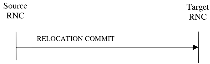
Figure 5: Relocation Commit procedure, Successful Operation
