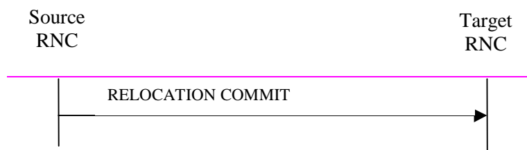
Figure 3: Relocation Commit procedure, Successful Operation
