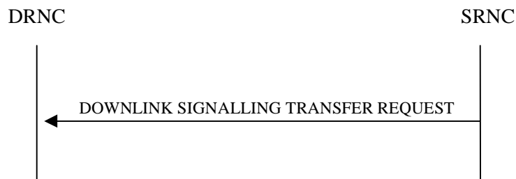
Figure 2: Downlink Signalling Transfer procedure, Successful Operation
