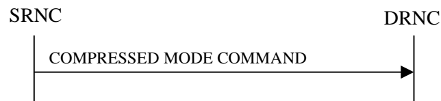
Figure 18: Compressed Mode Command procedure, Successful Operation
