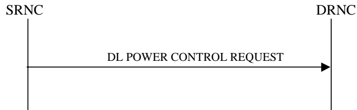
Figure 17: Downlink Power Control procedure, Successful Operation
