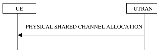
Figure 35: Physical Shared Channel Allocation
