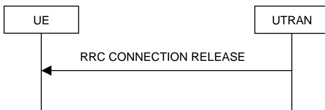
Figure 10: RRC Connection Release procedure on the CCCH
