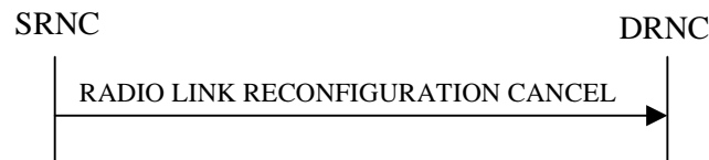
Figure 4: Synchronised Radio Link Reconfiguration Cancellation procedure, Successful Operation
