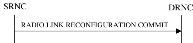
Figure 3: Synchronised Radio Link Reconfiguration Commit procedure, Successful Operation
