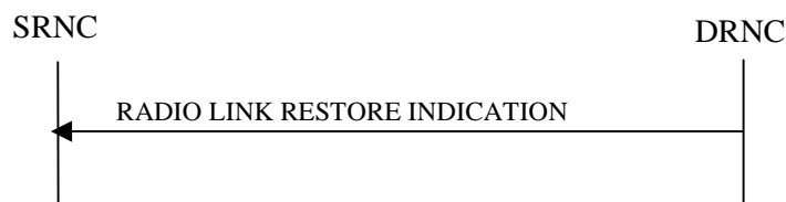
Figure 6: RL Restoration procedure, Successful Operation
