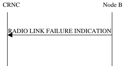
Figure 7: Radio Link Failure
