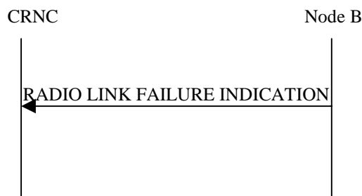
Figure 1: Radio Link Failure procedure: Successful Operation
