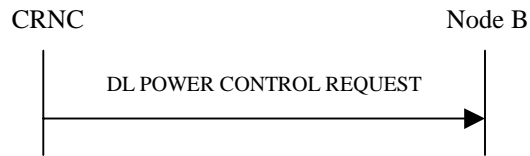
Figure 35: Downlink Power Control Procedure : Successful Operation
