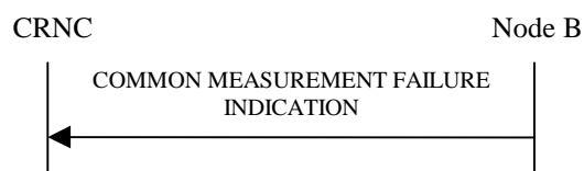
Figure 1545: Common Measurement Failure procedure: Successful Operation
