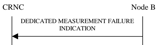
Figure 40: Dedicated Measurement Failure procedure: Successful Operation
