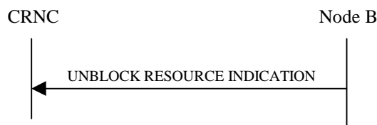
Figure 88: Unblock Resource procedure, Successful Operation
