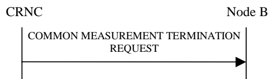
Figure 1444: Common Measurement Termination procedure: Successful Operation
