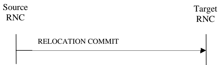
Figure 3: Relocation Commit procedure, Successful Operation
