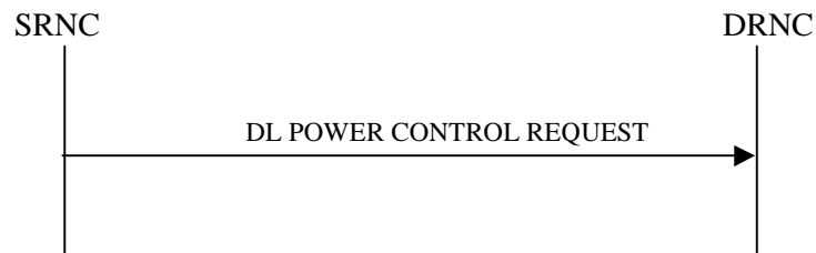
Figure 1: Down Link Power Control procedure, Successful Operation
