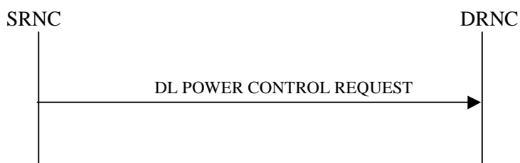
Figure 225: Down Link Power Control procedure, Successful Operation
