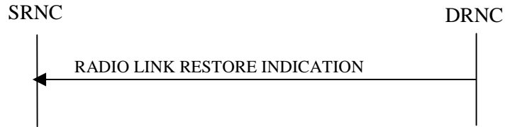
Figure 2: RL Restoration procedure, Successful Operation
