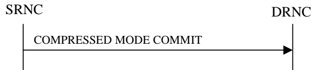
Figure 28: Compressed Mode Commit procedure, Successful Operation
