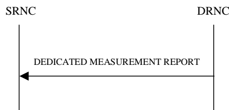
Figure 22: Measurement Reporting procedure, Successful Operation
