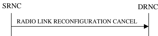
Figure 143: Synchronised Radio Link Reconfiguration Cancellation procedure, Successful Operation
