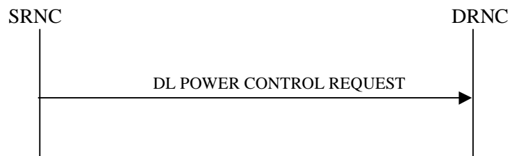
Figure 25: Downlink Link Power Control procedure, Successful Operation
