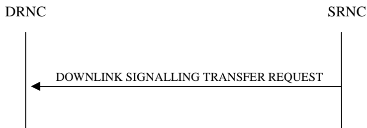
Figure 2: Downlink Signalling Transfer procedure, Successful Operation
