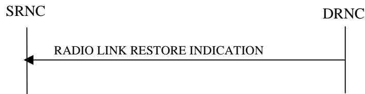
Figure 19: RL Restoration procedure, Successful Operation
