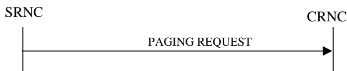
Figure 4: Paging procedure, Successful Operation
