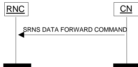
Figure 2: SRNS Data Forwarding Initiation procedure.
