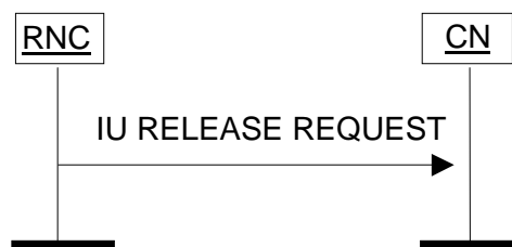
Figure 3: Iu Release Request procedure. Successful Operation.
