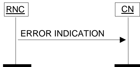
Figure 234: Error Indication procedure, RNC originated.
