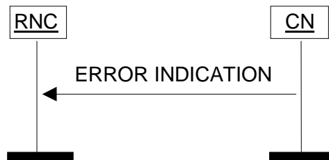
Figure 133: Error Indication procedure, CN originated.
