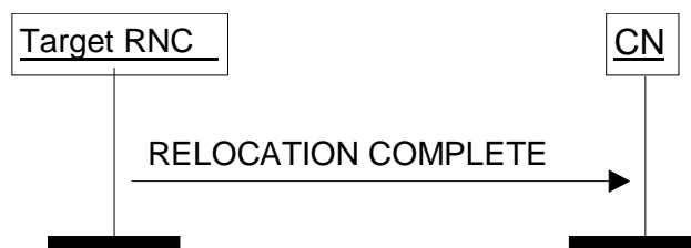
Figure 10: Relocation Complete procedure. Successful Operation.
