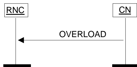
Figure 29: Overload at the CN.
