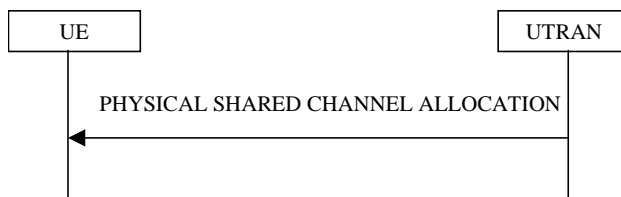
Figure 29: Physical Shared Channel Allocation
