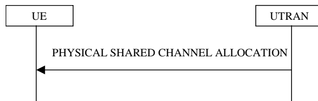
Figure 29: Physical Shared Channel Allocation
