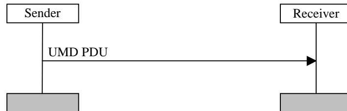
Figure 11.2: Unacknowledged mode data transfer procedure
