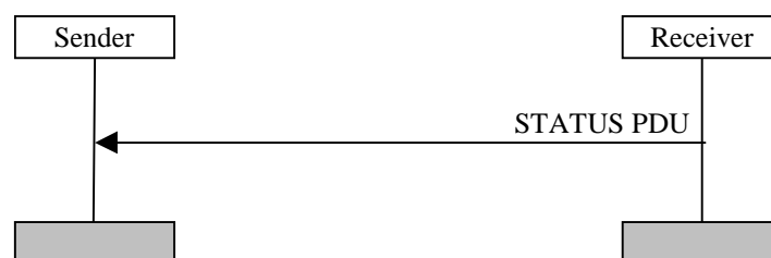
Figure 11.5: STATUS Status PDU report transfer procedure
