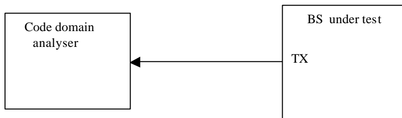
Fig.B.2 Measuring system Setup for CPICH power accuracy and peak code domain error measurements
