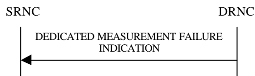
Figure 24: Measurement Failure procedure, Successful Operation
