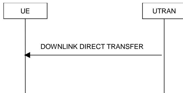
Figure 2. Downlink Direct transfer, normal flow
