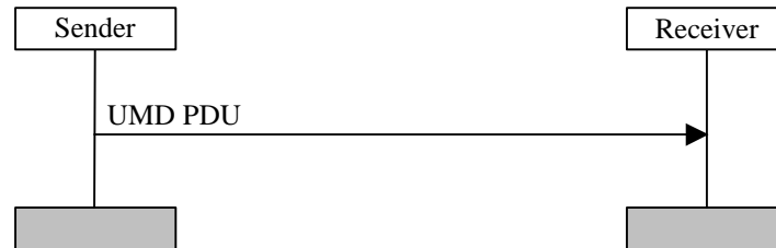
Figure 11-2. Unacknowledged mode data transfer procedure.
