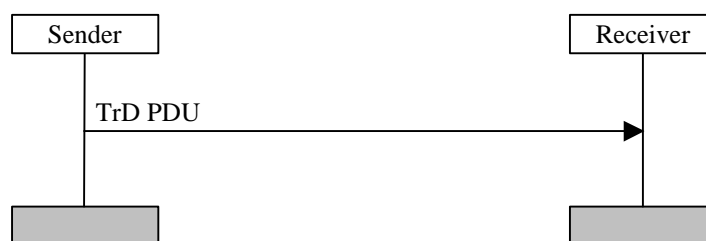
Figure 11-1. Transparent mode data transfer procedure.
