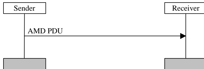
Figure 11-3. Acknowledged mode data transfer procedure.
