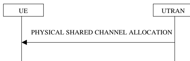
Figure 3128: Physical Shared Channel Allocation
