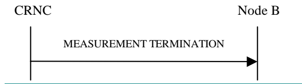
Measurement Termination Procedure initiated by RNC
