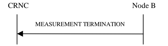
Measurement Termination Procedure initiated by NodeB
