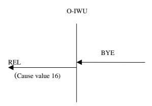
On receipt of a BYE method, the O-IWU sends a REL message with Cause Code value 16 (Normal Call Clearing).
