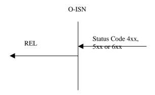
The reception of Status Codes 4xx, 5xx or 6xx will trigger the sending of a REL message. The coding of the Cause parameter value is derived from the Status code received according to table yy.
