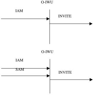
After initiating the normal incoming BICC/ISUP call establishment procedures, determining the end of address signalling and selecting to route the call to the SIP network domain, the O-IWU shall send the initial INVITE with pre-conditions. Only calls with Transmission Requirements of speech or 3.1kHz audio will be routed to the SIP network domain, all other types of call attempts will be rejected.
