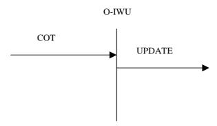
When the requested preconditions in the SIP network have been met, outstanding continuity procedures successfully completed and the incoming bearer establishment procedures (in the case of BICC) successfully completed, the UPDATE is sent confirming that all the required preconditions have been met.
