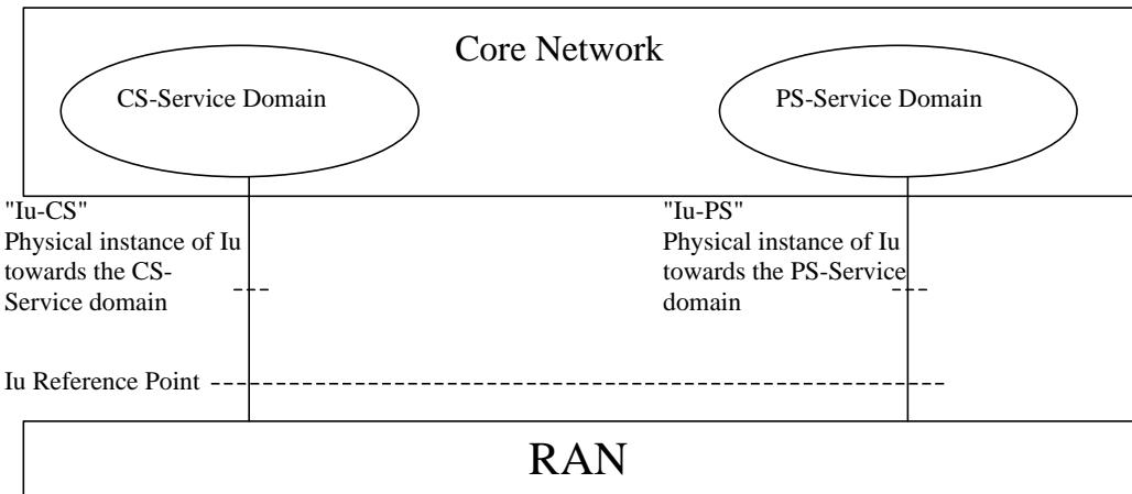
**Figure 1 - Ju Reference point, and the Ju-CS and Ju-PS physical instances**
