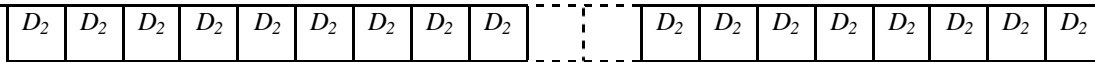
Figure 7: Example of OFDM 2-D structure; P = pilot or signaling, D = data. The subscript indicates the modulation level M=2,4 or 6 (QPSK, 16QAM or 64QAM).
